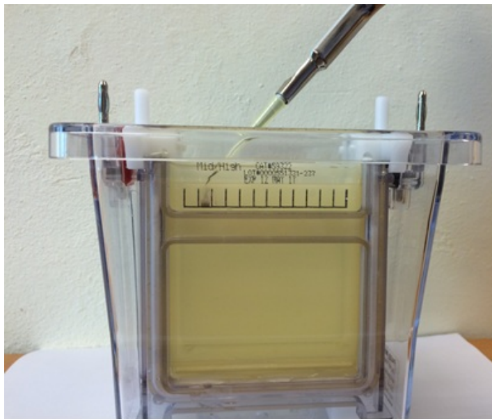
Fig.1.2. Sample loading on SDS gel
